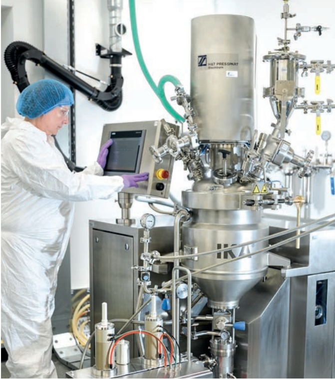
25L mixing vessel for development to pilot scale batches
